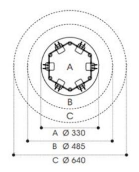
Due to its rocking function Hangaround needs about a meter of free space around it, which should be taken into account when placing the product in the space.
